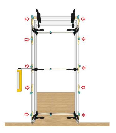
After the assembly foam has dried, try on the door leaf to the frame in the reverse order to disassembly.
