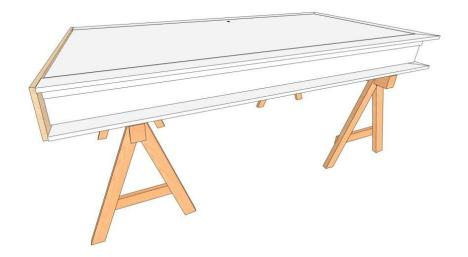
The door with the frame is factory assembled into a complete set, which facilitates preparation for assembly.
