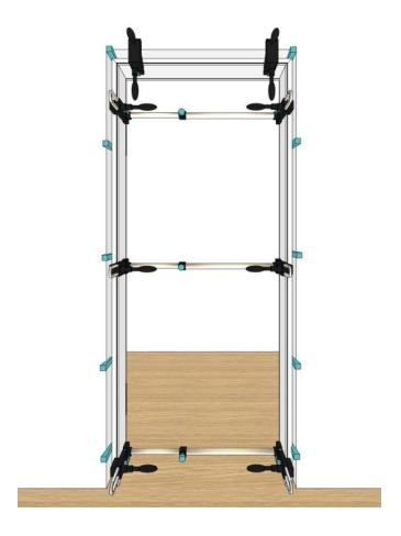
Check that the right angle is maintained between the frame legs and the top beam using an angular gauge.
