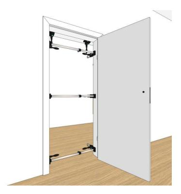
Check the gaps between the door and the frame. Perform a trial opening and closing of the door, checking that the lock and hinges work properly. Remove the door leaf.
