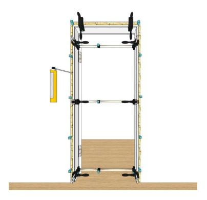
After the mounting foam is cured, install the door leaf. Adjust the hinges so that the gaps between the door and the door frame are the same on all sides
