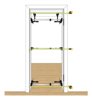
The linearity of the frame legs should also be checked. If necessary, adjust them using the clamps.
